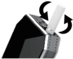
2:Sliding button to take out the cartridgeholder and take out the cartridge, and replace it with a new one.
